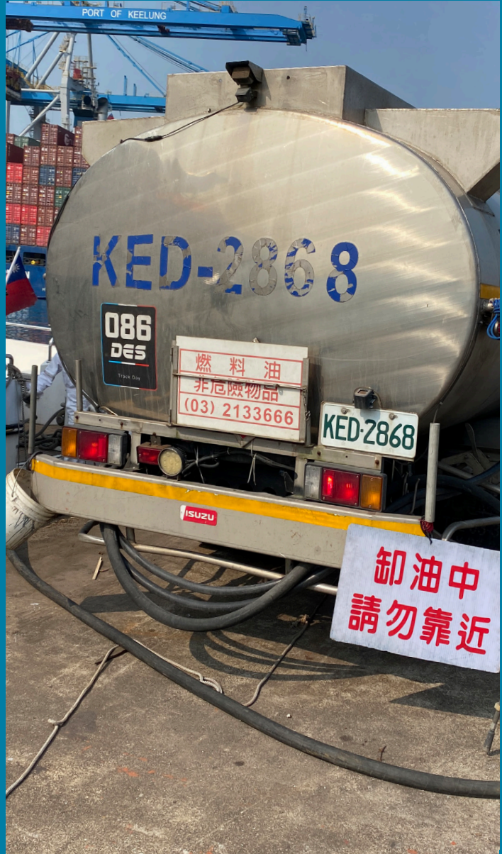
Tank Truck Fueling Operation for Ship (2,500 Liters of Ultra-Low Sulfur Diesel)
