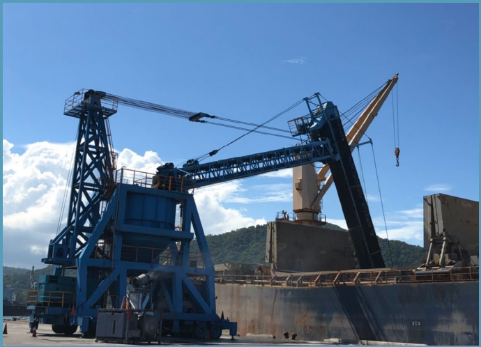
Port of Suao uses automatic coal unloading machine to reduce one of its main air pollution sources.
