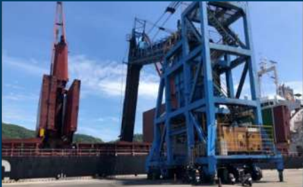
Automated coal unloaders and mist sprayers: enhance operational efficiency and reduce fugitive dust emissions
