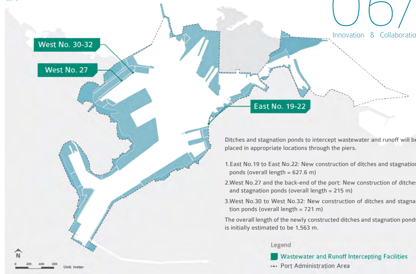
» Pier Locations for the Placement of Wastewater and Runoff Intercepting Facilities
