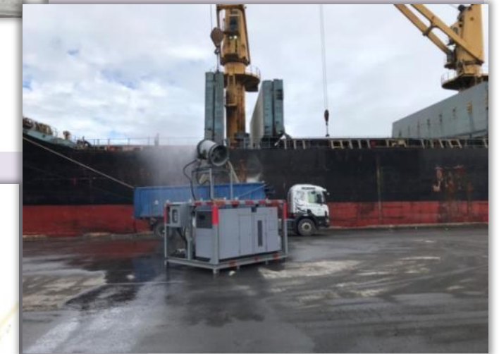
For the details of current onsite pollution preventive actions, there must be at least one water spray for every grabber to minimize dust. Furthermore, grabber shall not release the cargo until it reaches the bottom of the truck.
